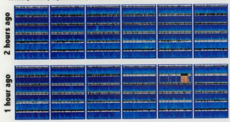
These spectrograms are computed by the IceWeb system using near-real-time data from the Iceworm system at the University of Alaska Geophysical Institute.
