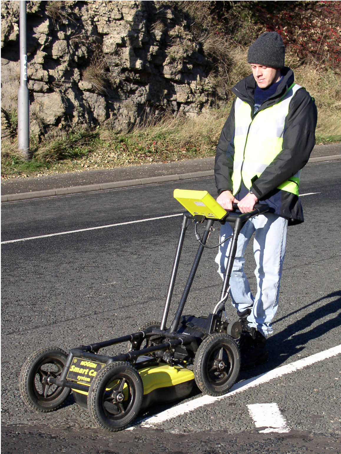
Figure 3 The geophysical equipment used in the survey. The ground penetrating radar unit is the black and yellow box seen between the wheels of the cart. This is connected to the yellow digital video logger.
