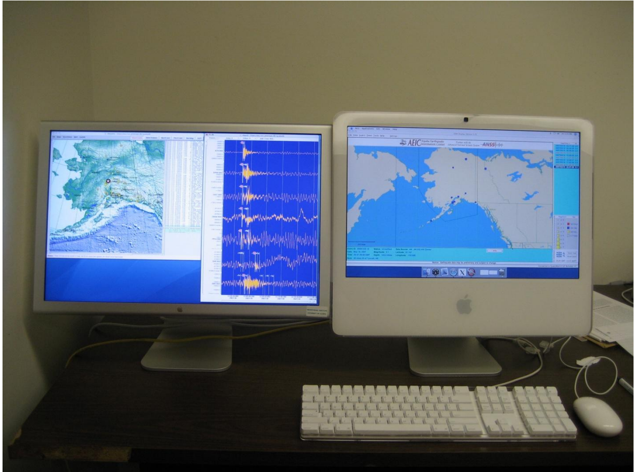
Figure 1: A photograph of the earthquake notification system. On the 23 inch monitor to the left the Antelope program dbevents_aeic is running. CISN_Display is running on the right monitor (this is actually the iMac computer with its integrated 20 inch monitor).
