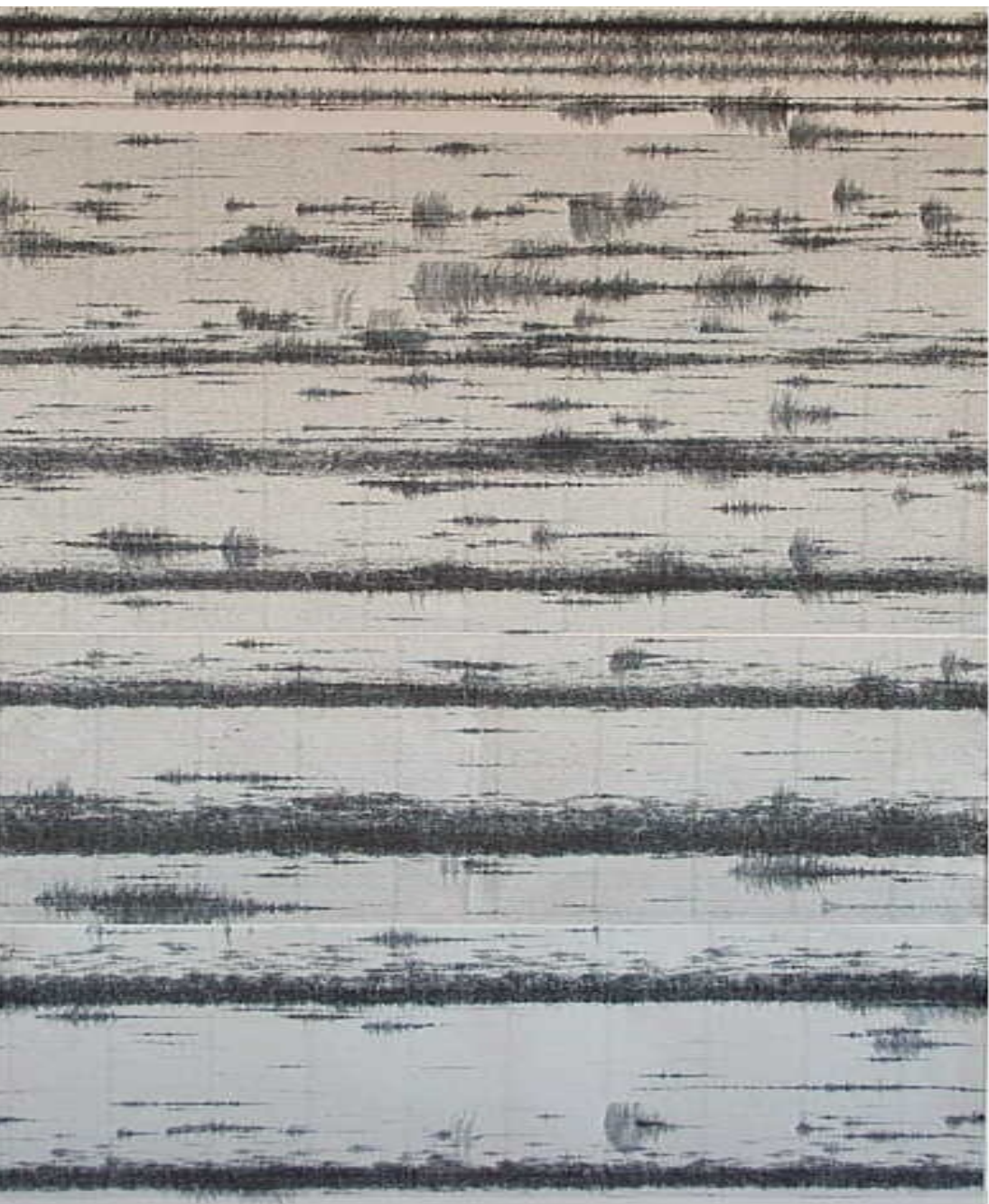
Figure 1: Banded tremor as it appears on a helicorder. This example is from 26 Feb 2001 – 1 Mar 2001, station MRYT.
